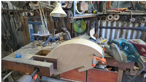
*All six formers clamped together to sand the curved faces for the jibs together.*
