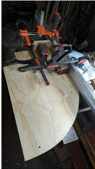
*Wooden blocks clamped and glued to the patterns in the register corner, to make it easy to clamp them to the stocks.*
