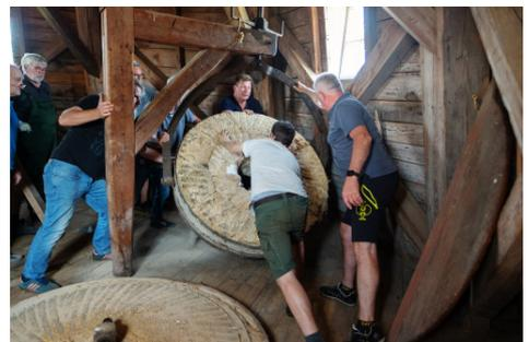
*A millstone crane is used to move the runner stone at Lübbertstedt Windmill.*
