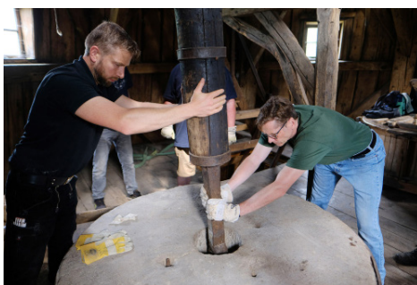
Björn and Silvio lower the quant inside the eye of the millstone.
