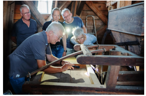
Johann Hüneke explains to his students the feeding shoe, crook string, the shoe handle and the damsel, at Lübberstedt Windmill in Northern Germany.
