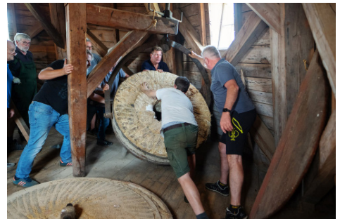
A millstone crane is used to move the runner stone at Lübberstedt Windmill.
