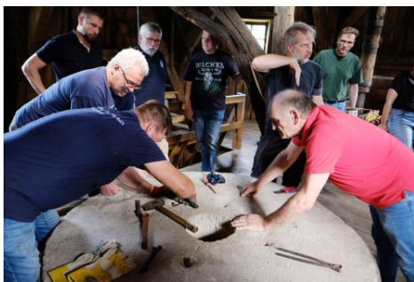
Preparations for lifting the runner stone inside a mill of the historic Museum Village in Cloppenburg.
