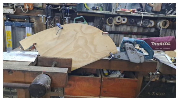
Sanding the six thin ply patterns clamped together.
