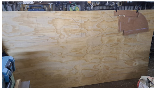
Marking out with the stencil made of hard-board, six times on thin plywood.
