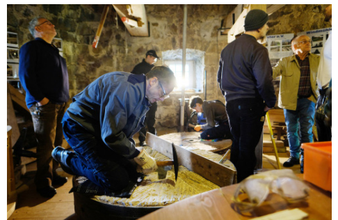
Silvio is dressing the bedstone at Exter Windmill. He uses a bill to carve out the furrows.
